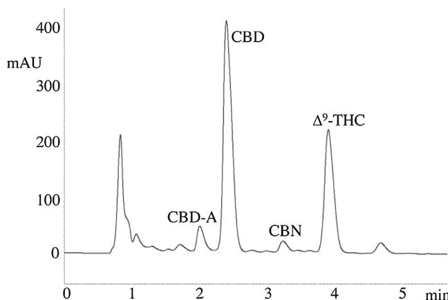
**Fig. 3.** Chromatogram referring to optimised conditions. Stationary phase, Agilent Poroshell® 120 SB-C18 analytical column. Mobile phase, mixture of ACN/5 mM K<sub>2</sub>HPO<sub>4</sub> pH 3.45. Flow rate, 0.38 mL min<sup>-1</sup>, temperature 53 °C. CBD-A, cannabidiolic acid; CBD, cannabidiol; CBN, cannabinol; Δ⁹-THC, Δ⁹-tetrahydrocannabinol.
